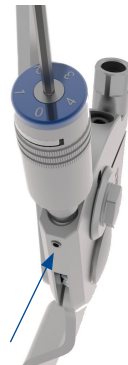
Figure 3. Loosen the ROM Dial screw using the 2mm adjustment wrench and zero the PF ROM setting by turning the blue ROM dial. The plantarflexion channel side of the component body serves as a reference for this adjustment.
