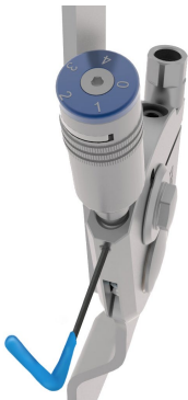
Figure 1. Unlock / lock the PF ROM Adjustment using the 1.5mm hex wrench to loosen / tighten the ROM Lock Set Screw.
